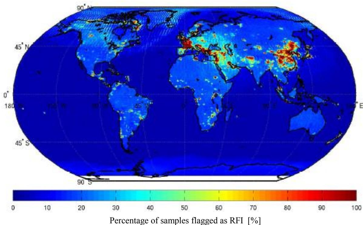
Fig 1. Percentage of Aquarius samples flagged as RFI for one year (August 25, 2011 to August 25, 2012. This is the average of observations at both horizontal and vertical polarization.
